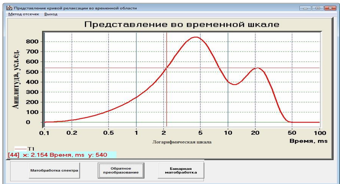
Figure 4.6 – Spectral representation of T1 longitudinal relaxation times obtained by NMR measurement of rock sample No 111
